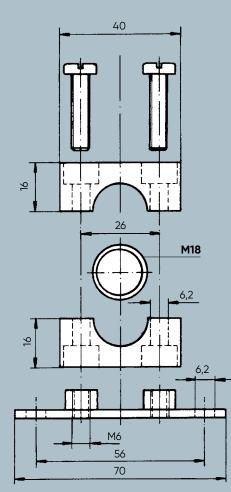
Width of the weld-on plates: 30mm Thickness of the weld-on plates: 7 mm
